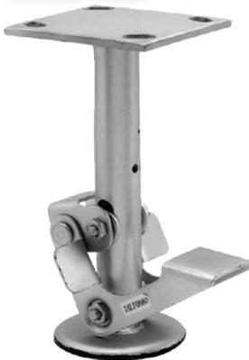
Designed to hold portable equipment in a desired location. Intended for use on level surfaces. Floor lock is activated by toe pressure on the extension pedal or released by toe touching one of the dual retractable plates. The large non-skid brake pad, under high spring compression, holds the portable piece of equipment until released. For best results, units should be used in pairs.
