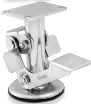
The Albion 02 Series floor locks are designed to hold your portable equipment in a desired location. Intended for use on level surfaces, the floor lock is activated by toe pressure on the extension pedal or released by toe touching one of the dual retractable plates. For best results, units should be used in pairs.
