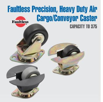
Designed for inverted applications, these Faultless conveyor casters are designed for easy installation and replacement in the field. Special dust-and-grease cap and special all-temperature lubricant are standard along with precision bearing swivel and needle bearing wheels. Corrosiveresistant zinc dichromate finish is standard.
