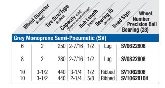
The SV wheel provides you with all the benefits of a pneumatic tire, without the hassle of getting a flat. These maintenance free wheels, constructed of solid monoprene material, which rejects debris and will not go flat, offer the same great features of a pneumatic wheel.
