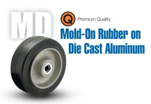
Cushion rubber treads are vulcanized to die cast aluminum core. The soft rubber tread affords a cushion effect to the load and excellent floor protection. These wheels are highly shock absorbing and provide quiet operation, while dampening vibration.
