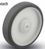
TPE HI-TEMP wheels are perfect when you need an economical alternative for moderately high temperature environments. The wheels are crafted of grey thermoplastic elastomer tread chemically bonded to a white polyolefin core and feature a single insert molded stainless steel radial bearing. TPE HI-TEMP are ideal for medical applications and environments requiring wash down.
