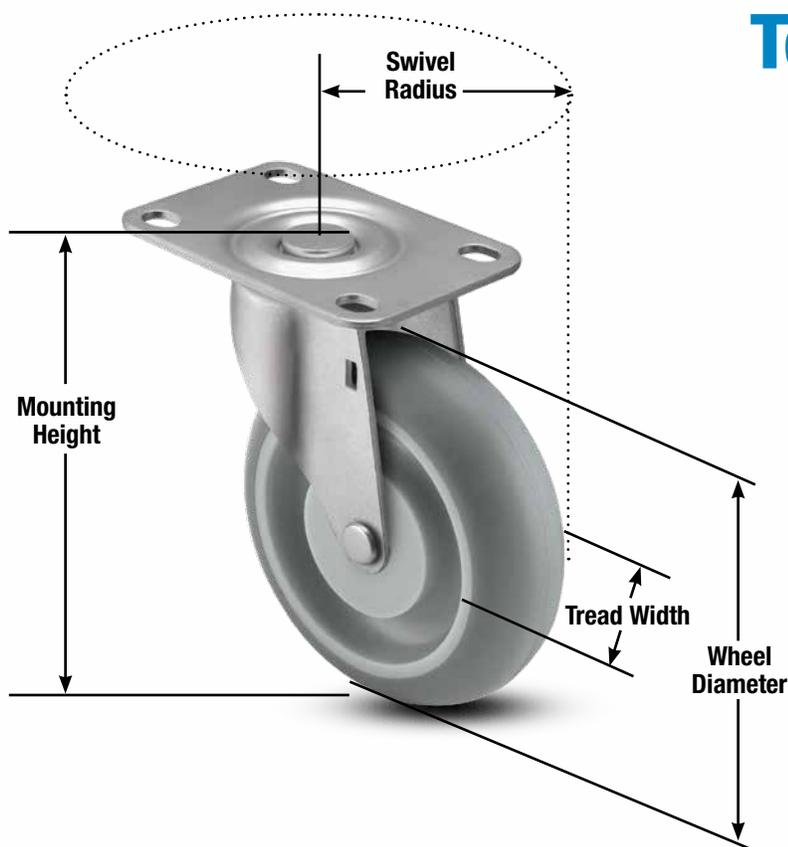
**Swivel Radius** – The distance from the center of the fastening to the outer most point of the caster. This specifies the minimum clearance required for a mounted caster to swivel 360 degrees.
