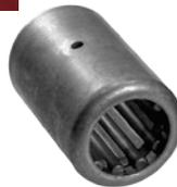
These are roller bearings as described above except they have metal cages holding the precision ground rollers. The outer race is a one-piece construction, giving added rigidity to the wheel bore. These bearings must be used on a hardened bushing or shaft. Maximum temperature range is 400°F.
