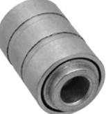
A precision type bearing where the machined outer race and inner race are held together by the bearings. This option offers easy rolling and quiet operation for light to medium duty loads. This bearing must be factory installed in the wheel. Designed for temperatures up to 160°F.
