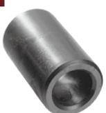
This is a one-piece version of the Delrin bearing listed above. Good for use where thrust washers are needed or to add rigidity to a soft wheel which might cause the two piece bearing to be ejected from the bore of the wheel. Maximum temperature range is 160°F.
