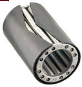
Roller bearings are the standard bearing in most caster applications. 1-1/2 and 2 inch width wheels feature a cage separating hardened steel rollers and a hardened steel split outer race. These bearings must be used on a hardened bushing or shaft. Maximum temperature range is 350°F. All Casters and wheels are rated up to 2.5 mph operation per the Institute of Caster & Wheel Manufacturers Guidelines.
