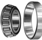
The tapered roller is the most effective bearing for heavy or towed loads. The taper allows for some thrust loading, while the heat-treated inner and outer race allow for maximum load capacity. Maximum temperature range is 400°F.
