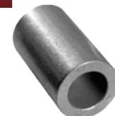
These bearings are made of oil-impregnated sintered iron. Completely self-lubricating, these are ideal for situations where rolling force is less critical and accessibility for lubrication is difficult. Maximum temperature range is 450°F.
