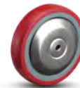
Hi-Temp Thermal Rubber (ARZ) Antimicrobial wheel. Stainless steel thread guards standard. 280 degrees Wash down (10 minutes), Auto Clave / Steam Sterilizer instrument wash @ max load of 90kg per wheel under heat and 108kg at room temp. Durometer: 78-85A
