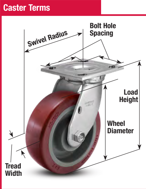
Photo above shows typical wheel. Bearings, bushings, etc. may vary with different wheel types.
